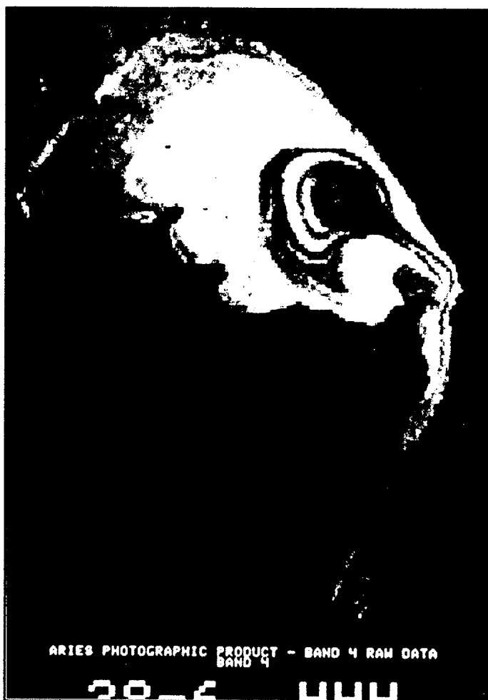
Figure 14 Satellite Image of Oil On Ice in Gabarus Bay, Streaks in Centre of White Ice Patch Are Oil, Outer Material is Sediment
