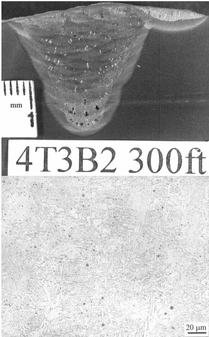
Figure 45: Macro-section and top bead microstructure from 4T3B2 V-groove weld.
