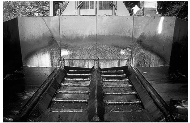
FIGURE 15-5 Slat conveyors at bottom of paver hopper.
