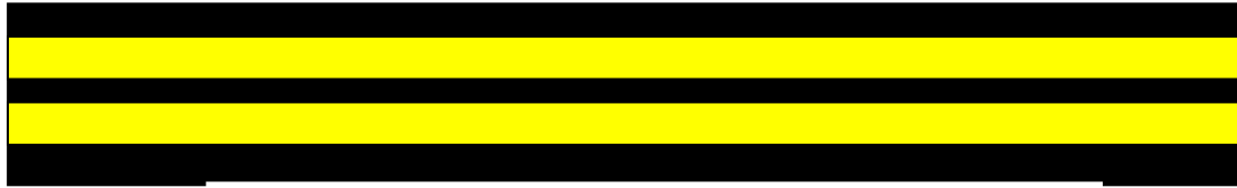
Figure B-3. Continuous Taxiway Edge Line Marking
