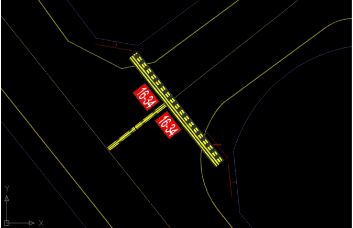
Figure C-12. Intersection of Stub Taxiway and Runway
