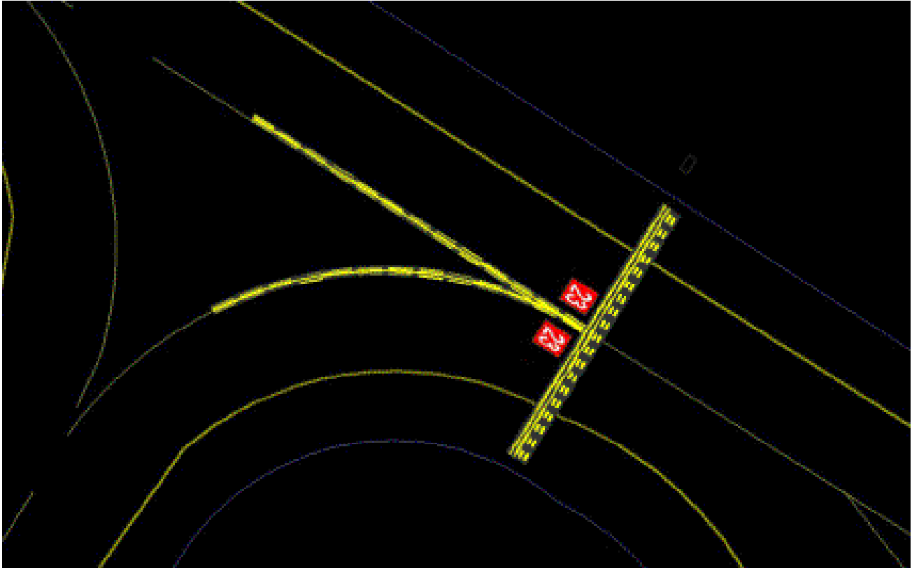
Figure C-8. Intersection of Two Taxiways at Runway End
