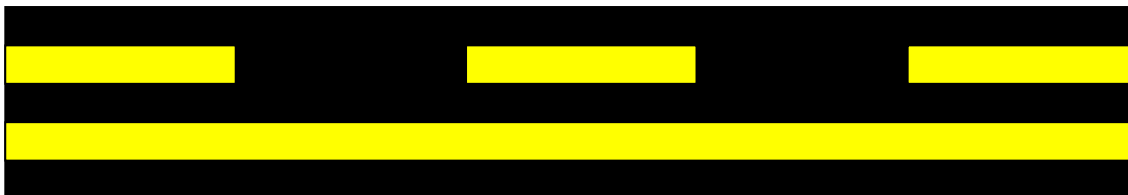
Figure B-8. Non-movement Area Boundary
