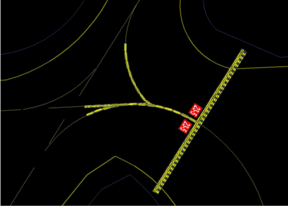
Figure C-9. Intersection of Three Converging Taxiway Centerlines
