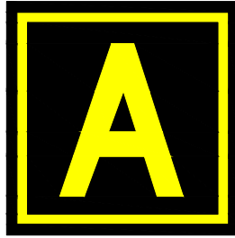
a. Taxiway Location Sign
