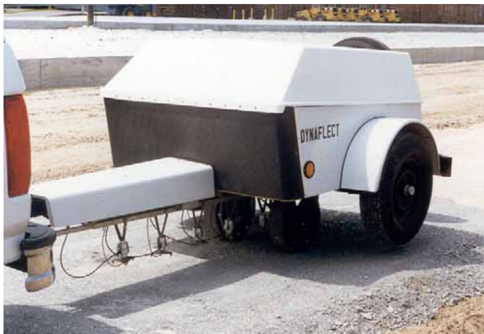
FIGURE 8. DYNAFLECT DEFLECTION TRAILER
