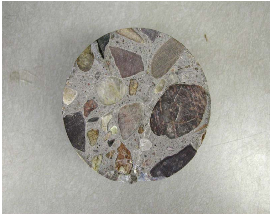
Figure 3-1. A slice of a concrete core collected from an airfield pavement under plain light (scale: 1= 1.75).
