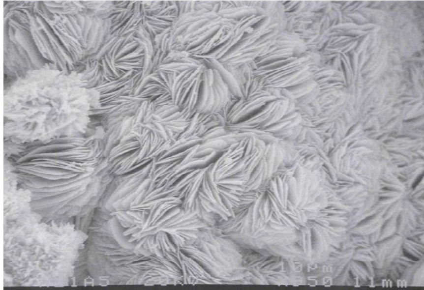
Figure 3-10. SEM image of rosette like crystalline ASR gel product.
