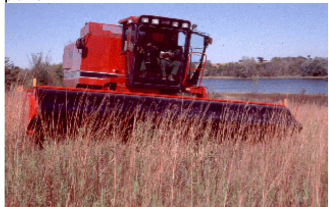
This prairie grass combine harvests the seeds while leaving the grass stems standing for winter cover and spring nesting habitat.
