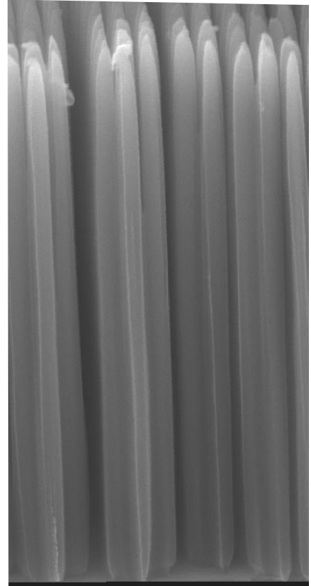
This image is a scanning electron micrograph of tall (35:1 aspect ratio), closely packed, well-defined, 200-nm-diameter pillars etched with ENABLE into a polyimide film using nanospheres as a shadow mask.
