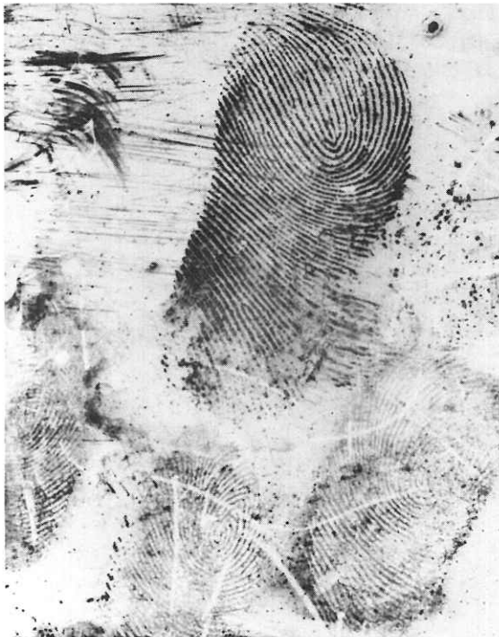
The fingerprints on this plastic credit card were developed by the Universal Process.
