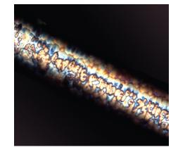
Shown is an image of a boron-carbonsilicon alloy fiber grown by highpressure laser chemical vapor deposition using a very small laser spot. The fiber was grown at 10 cm/s and shows no cracks or fracture planes that can compromise the entire structure.
