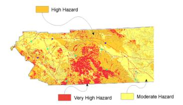
This map indicates moderate, high and very high hazard based on inputs, such as fuel, slope, brush density (ladder), and tree density (crown cover).
