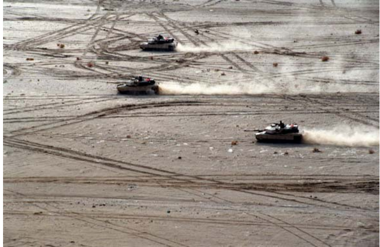
Tank maneuver area is permanently non-vegetated. Runoff from these areas must be managed through LID IMPs surrounding the area.
