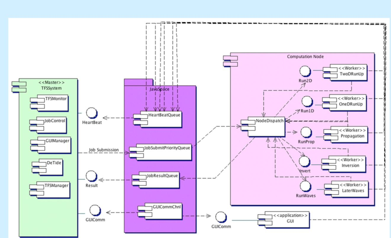
The system has a modular design with a robust cross-platform architecture. The primary programming language is Java (J2SE5.0) with Jini 2.1 technology for network services. The models are written in Fortran 77. Development is performed in JBuilder using Java coding standards with JUnit testing. Subversion 1.2 is used for configuration management.
