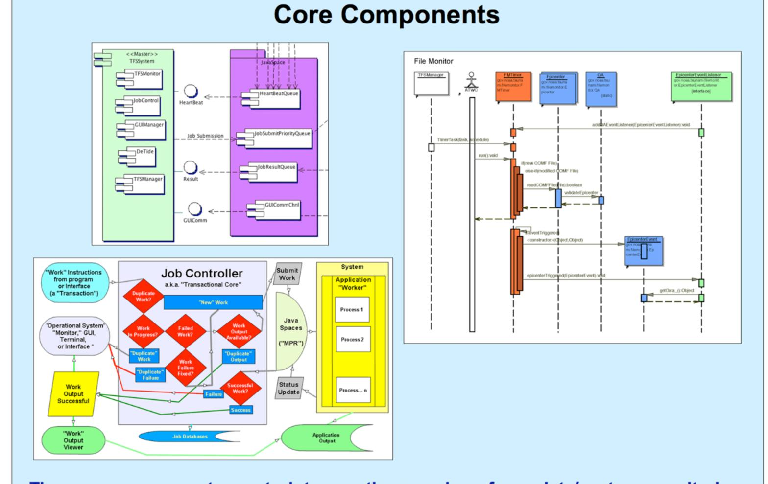
The core components control transactions and perform data/system monitoring. JavaSpaces are used to communicate between different components. A PostgreSQL relational database is used to manage jobs, data, and configuration parameters.
