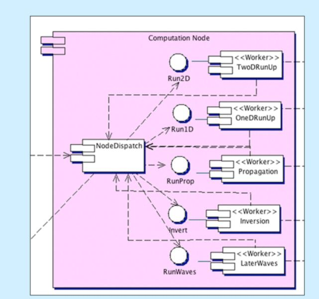
The first version of the system will include the propagation node, which uses pre-computed model runs of unit tsunamigenic sources. The data are stored in netCDF files, with metadata stored in a PostgreSQL database.
