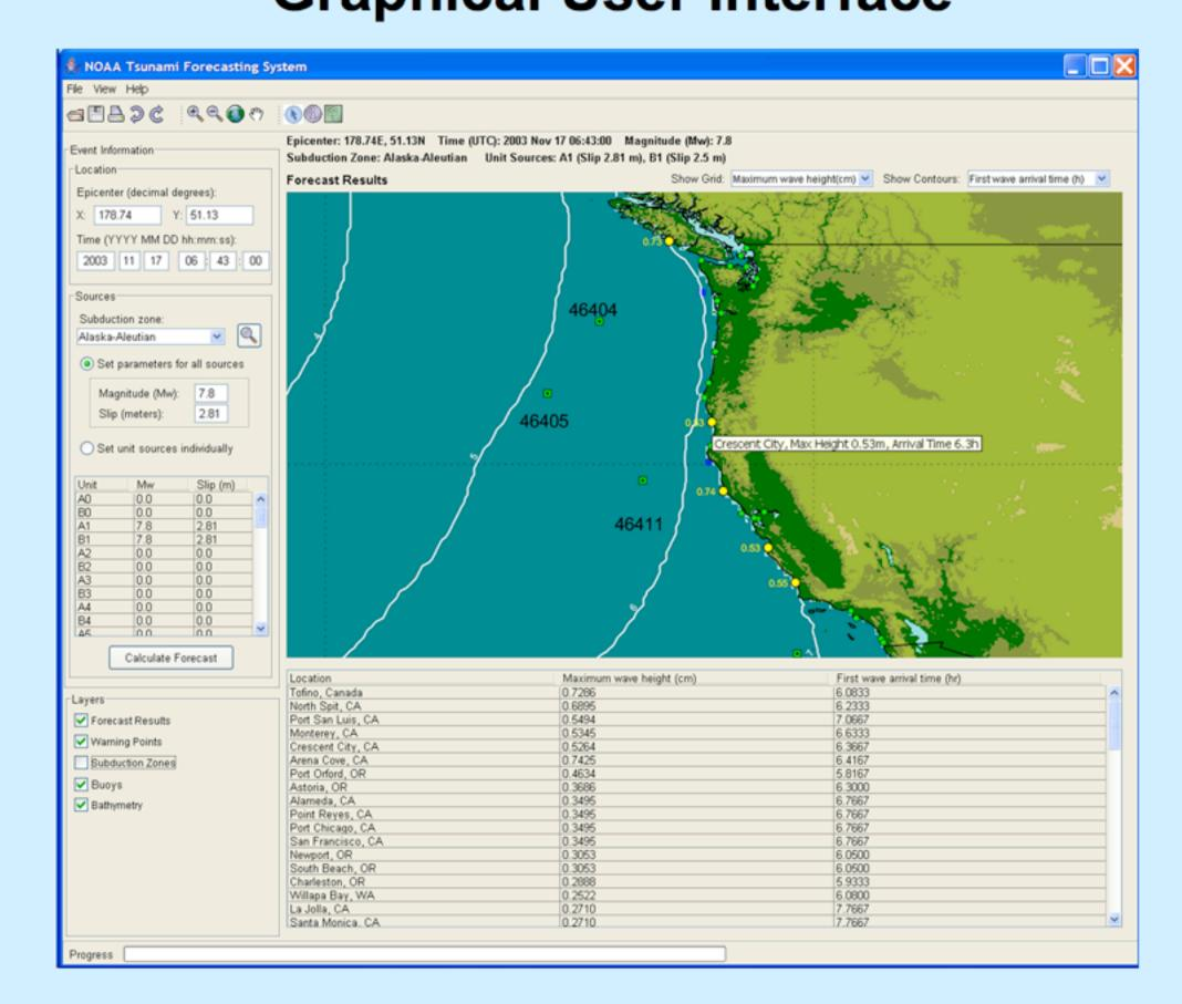
The GUI is designed for easy access to model results with minimal user input. Offshore and coastal forecasts can be generated automatically or based on user input. The design will be modified based on usability requirements and tests from both Tsunami Warning Centers.
