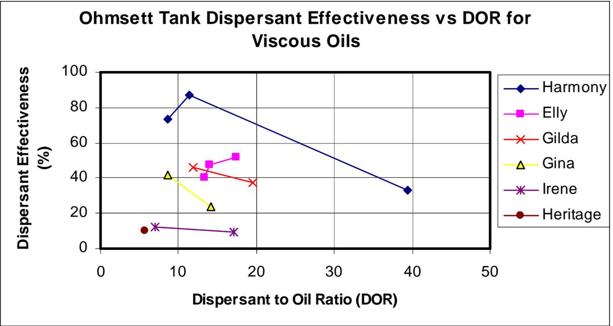
Figure 4. Ohmsett Test Tank Results: Dispersant Effectiveness versus DOR by Oil Name
