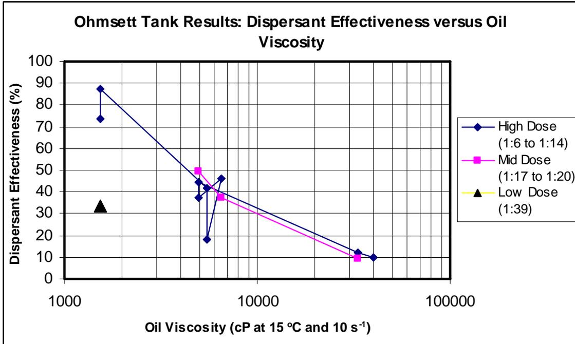
Figure 5. Ohmsett Test Tank Results: Dispersant Effectiveness versus Oil Viscosity
