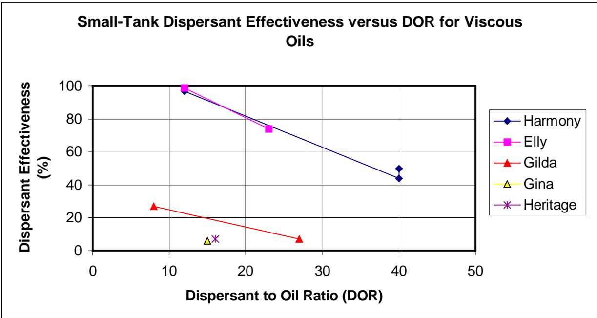
Figure 2. Small-Scale Tank Test Dispersant Effectiveness versus DOR by Oil Name
