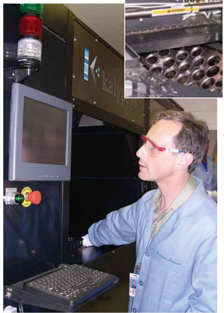
Hugh Fisher of Molecular Microbiology and Immunology (B-1) loads bacteria samples into the robot at a recent training session at the Health Research Laboratory. Inset photo: The centrifuge rotor is located inside the robot apparatus. It holds 96 tubes; the centrifuge alone weighs about 160 pounds. Photos by McIntosh
