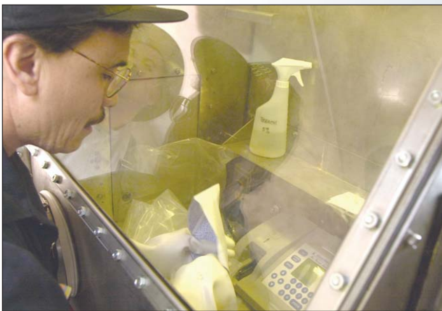
Using a sealed glove box, Robert Trujillo of Sandia National Laboratories analyzes an envelope that contained a powder substance at the New Mexico Hazmat Challenge. The scenario involved a letter with a suspect substance found inside a building. Trujillo is conducting a bio-threat-alert test. The glove box, which the Lab built and owns, can be used to test for a number of unknown substances.
