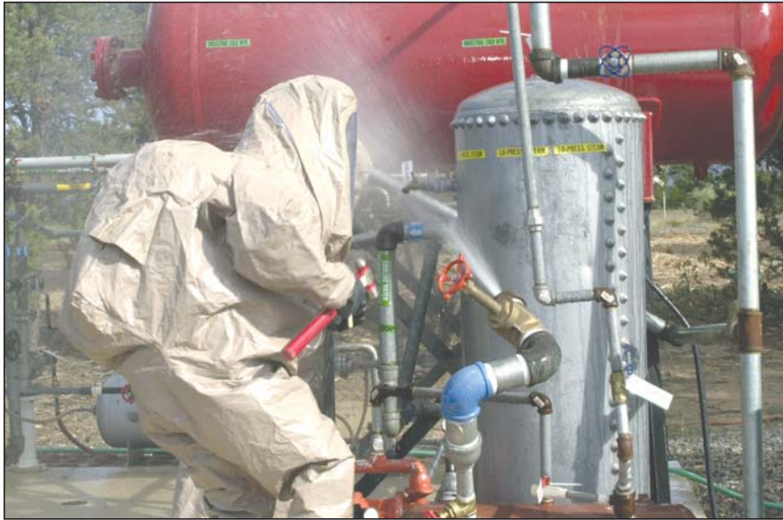
Members of the New Mexico National Guard team work to mitigate a leak in the valve/pipe tree at the 2002 New Mexico Hazmat Challenge at Technical Area 49. In this scenario, the team is responding to a pipe leak from an industrial accident.
