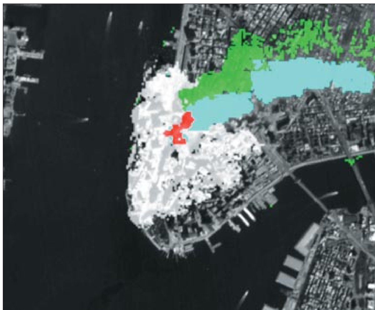
Feature-extraction algorithms (GENIE) were developed and applied to multispectral imagery of lower Manhattan post-Sept. 11. GENIE is a product of the Nonproliferation and International Security (NIS) Division. Here, GENIE identifies debris plume rising from the terrorist attack.
