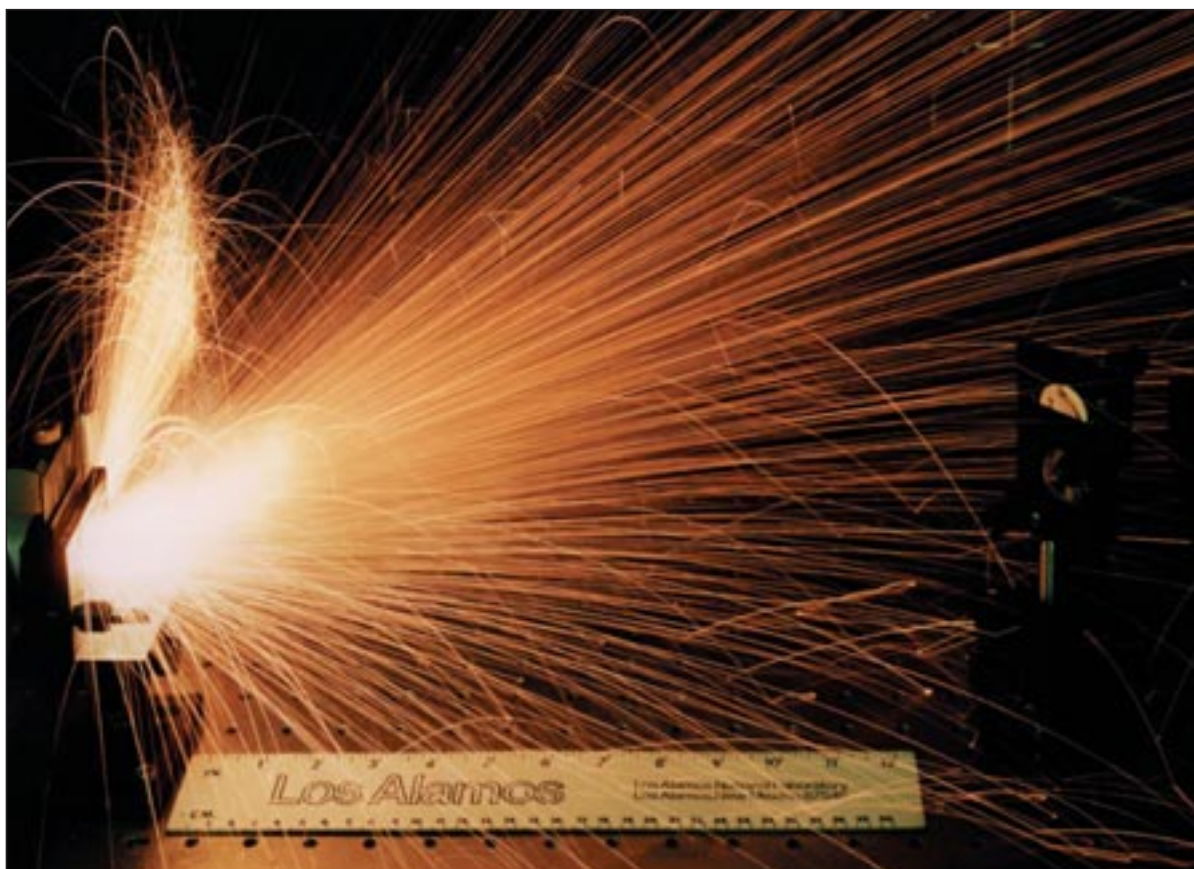
Metastable Intermolecular Composite (MIC) SuperThermites are a new class of energetic materials, discovered and developed at Los Alamos in the Dynamic Experimentation (DX) Division. MIC reactive fragments can carry both kinetic and chemical energy to the target. Chemical energy provides order-of-magnitude increased power over purely kinetic material.
