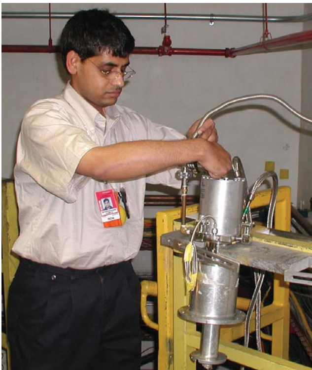
Siva Chinta from Texas A&M University's Department of Chemistry loads a sample of gold/titanium oxide into a closed-cycle refrigerator during the successful 2001 run cycle at LANSCE. Chinta used the Filter Difference Spectrometer at the Lujan Center to study the catalytic oxidation of propene on nanoparticles of gold on titania.
