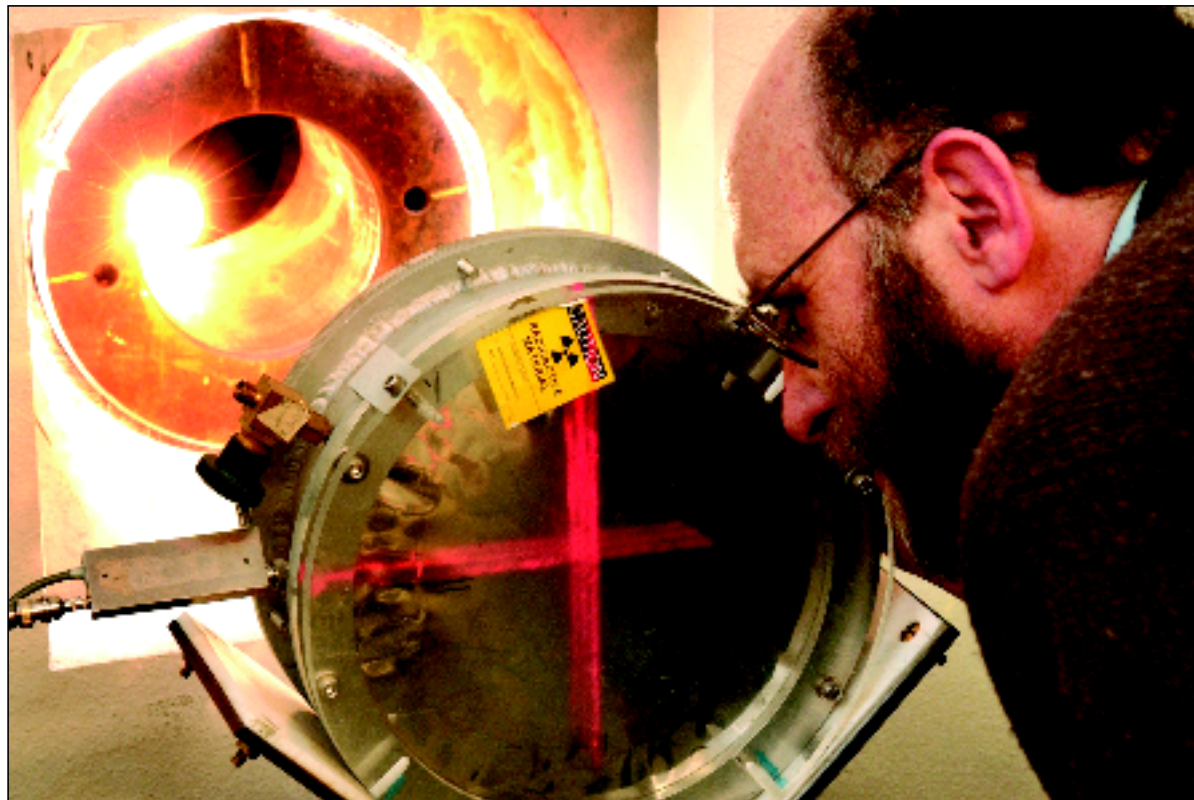
Steve Wender of Neutron and Nuclear Science (LANSCE-3) adjusts the fission ion chamber that is used to measure the number of neutrons that pass through it to the devices that are being tested. When the neutrons pass through the chamber, a fission reaction is detected and a signal is generated that is used by the experimenters to determine the number of neutrons that strike their devices. Photo by LeRoy N. Sanchez
