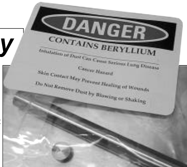
Small beryllium shapes, like this rod and pellet, are used to demonstrate the look and feel of engineered parts made from machined pure beryllium.
