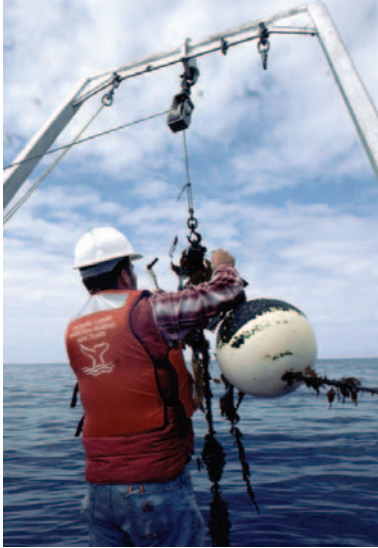
One of the buoys used to mount sensors. Photo: NOAA
