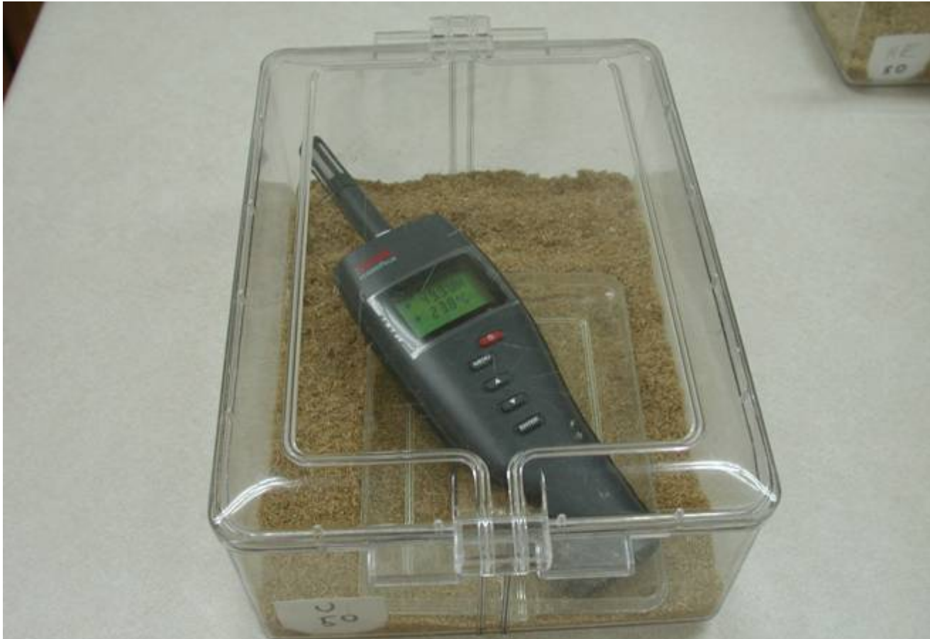
Hygrometer measuring water activity ( A_w ) of seeds in a covered box
