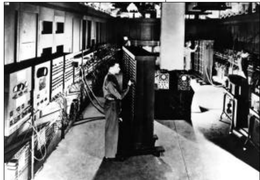
ENIAC, the first large-scale electronic computer, provided a calculation needed for the “Los Alamos problem.”
