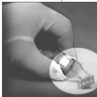
A short segment of a thick-film superconducting tape flexed around a spool. The tape delivered record current levels at relatively high temperatures.
