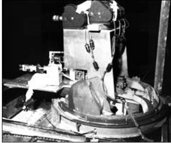
Berlyn Brixner sat in an observation bunker behind the 35mm Mitchell camera and four 16mm Kodak Cine E cameras mounted on the pivotal turret shown in the top photo; the lower photo shows 13 of the 37 motion-picture cameras used to film the test.
