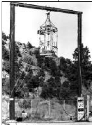
Lady Godiva — so named because her uranium core was unclad, as was the woman in the legend.
