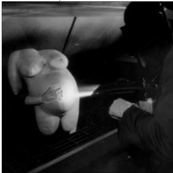
↑ Los Alamos researcher Richard Castro sprays a fine mist of nickel on an aluminum cast of the sculpture.
