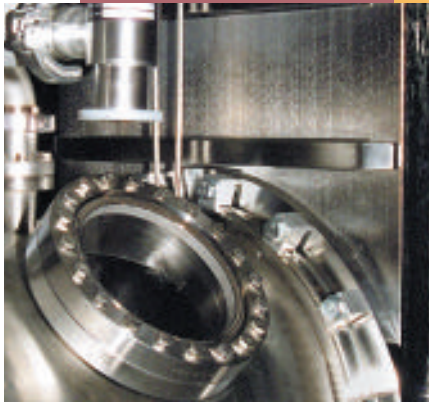
The airlock and part of the conveyor that integrate the ARIES modules.
