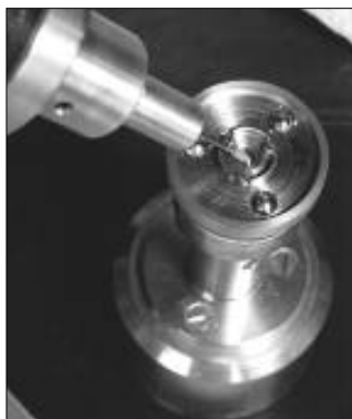
A close-up view of a Quick-Flip Locator attached to the spindle of a polishing machine.
