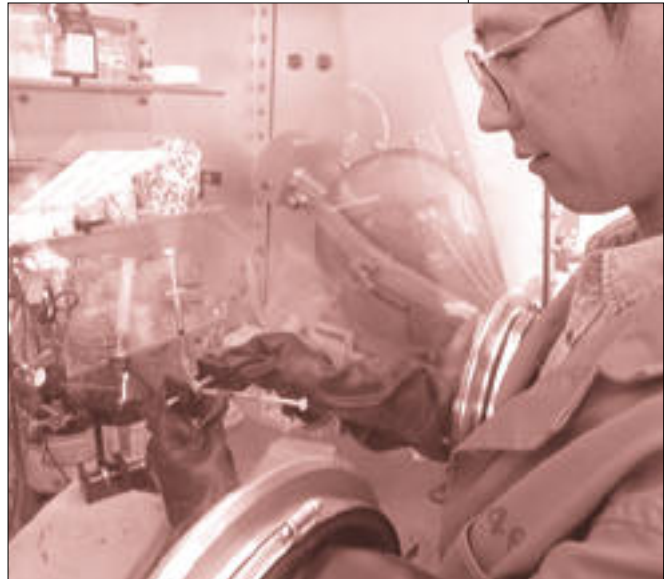
Researcher Steven Shi tests an ultracapacitor cell in a glovebox.
