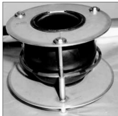
A bowling ball demonstrates a holding fixture for use in a pit storage container.
