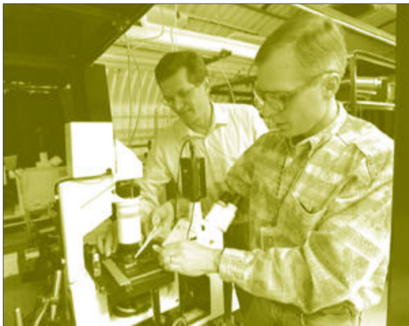
George Havrilla (left) and Jon Schoonover set up the Raman imaging microscope to analyze a sample.
