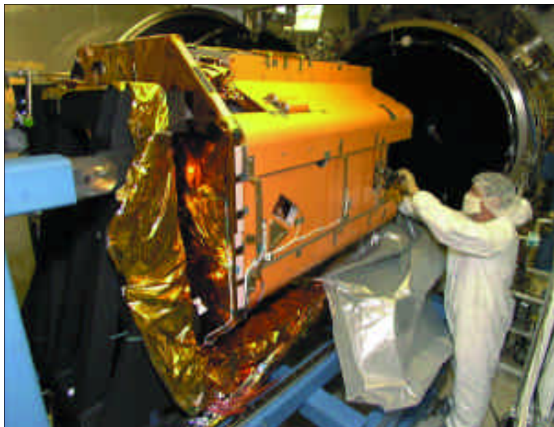
Bill Atkins rolls the satellite out of the thermal chamber during calibration last year at Los Alamos.
