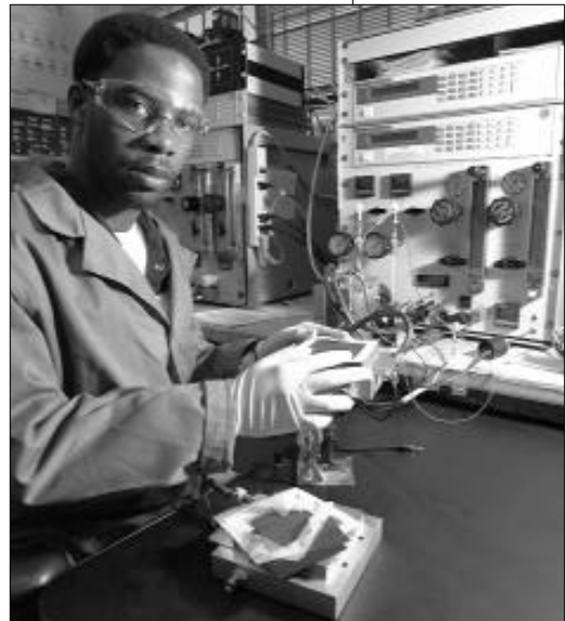
Tommy Rockward, a graduate research assistant, runs a test at a fuel cell testing station. He is collecting data to help determine the effects of impurities in the fuel stream on fuel-cell performance.
