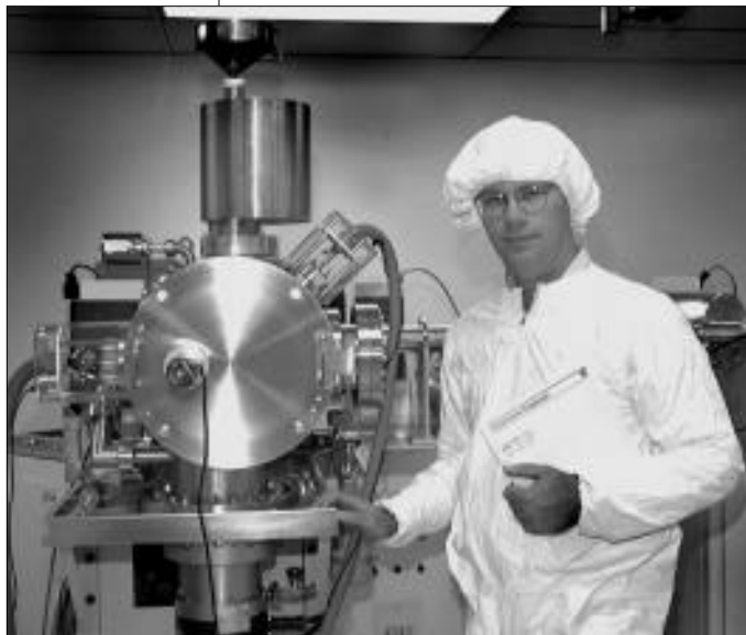
↑ Los Alamos researcher Steve Goldstein in front of a thermal ionization mass spectrometer.
