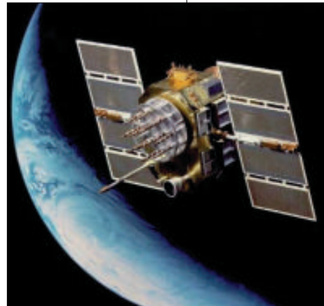
Global Positioning System satellites carry sensors that can pinpoint nuclear weapons tests anywhere in the world.
