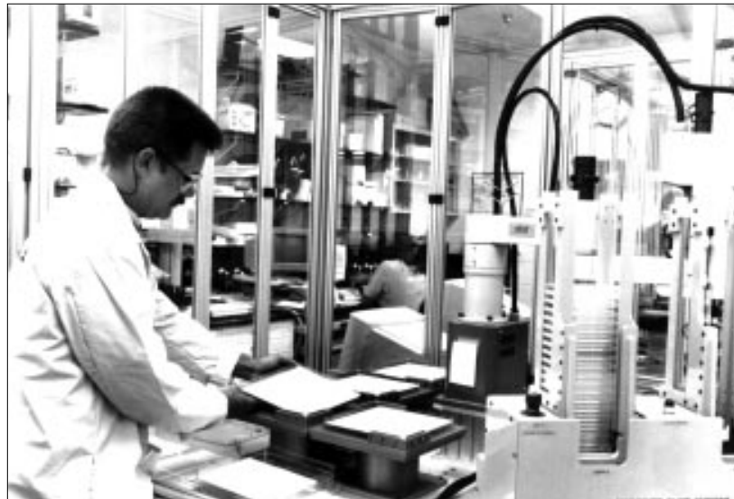
Los Alamos researcher David Bruce prepares a gridding robot for its designated task of transferring bacteria cells cloned for known fragments of human DNA from their storage sites to specific locations on a grid. By dipping the grid in a chemical bath containing DNA tagged with fluorescent dye, researchers can probe the grids for specific genes.
