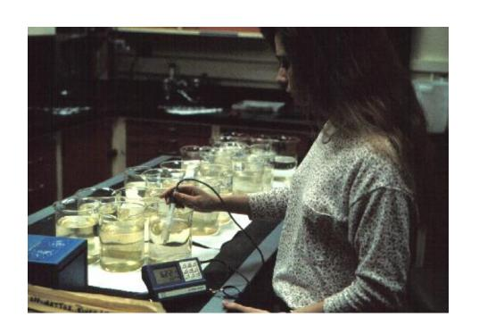
Analysis of Water Column Bioassay Test to Compute Toxicity (LC50) of CDF Effluents
