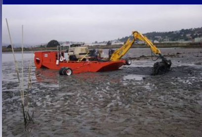
Aquamog: an underwater rototiller Aquatic Environment, Concord, CA
