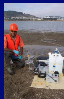
Water sampling above treatment plots at high tide
