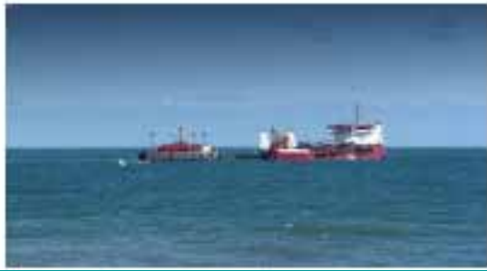
Offshore dredge used to pump sand for beach nourishment
