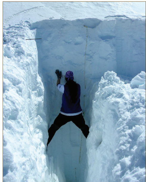
A researcher collects snowpack samples from the sides of the snow pit, avoiding contamination.
