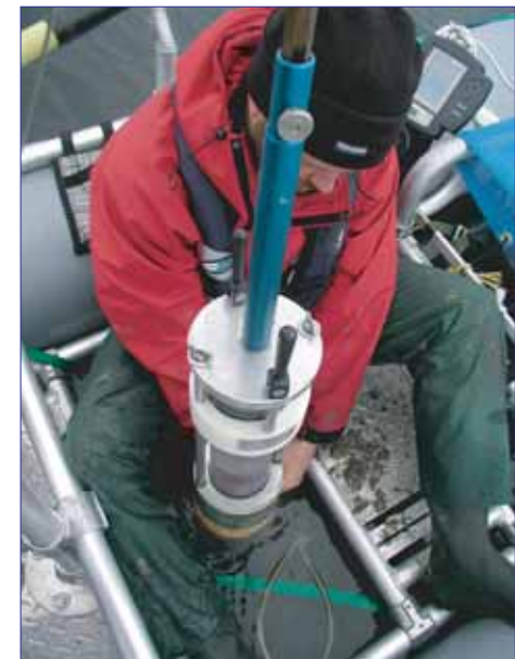
Figure 4. A scientist prepares to remove a successfully collected sediment core from the coring device suspended over the open-bottom sampling bay of the inflatable research raft on Burial Lake, Noatak National Preserve, in arctic Alaska.
