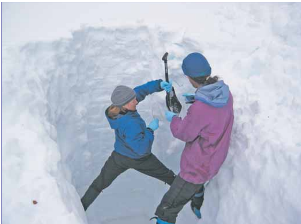
Figure 2. National park natural resource specialists sampling snowpack in Mount Rainier National Park in 2003. Samples are obtained from the vertical sides of a snow pit using clean field techniques to avoid contamination.
