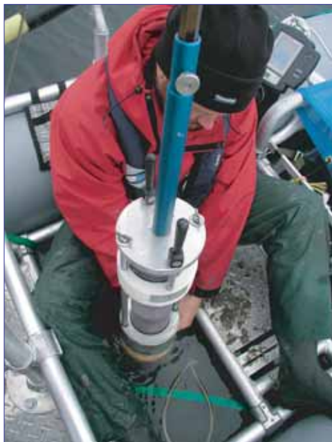
Figure 4. A scientist prepares to remove a successfully collected sediment core from the coring device suspended over the open-bottom sampling bay of the inflatable research raft on Burial Lake, Noatak National Preserve, in arctic Alaska.
