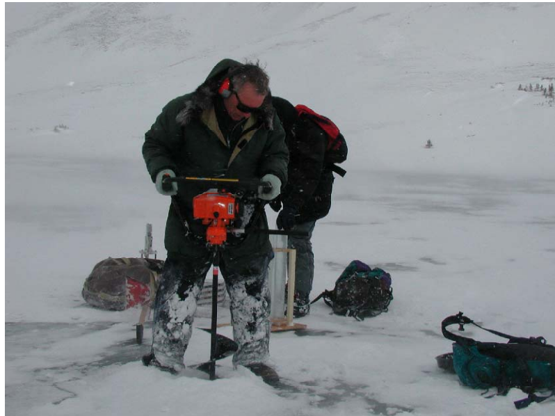
Figure 5.1 Drilling a 10 inch diameter hole in the ice is accomplished using a gasoline powered auger. Ice is usually from 1 to 2 meters deep at high elevation and or high latitude lakes.
