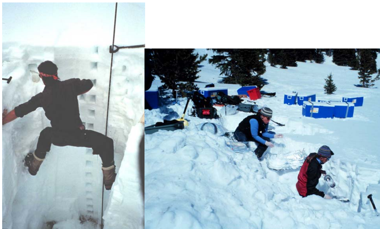
Figure 2.3 Snowpit physical profile and sampling for organic compounds
