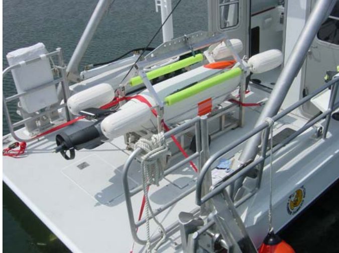
Figure 1. The Fetch 3.5 AUV on the back deck of SWFSC/AST's R/V D.V. Holliday during acceptance trials. The AUV includes a 38 kHz split-beam echo sounder, stereo imaging cameras and strobe, a CTD, Doppler velocity log, GPS, and 900 MHz ethernet telemetry. The AUV was tested off San Diego from July to December, 2005. Since then, procurement issues have halted its use.
