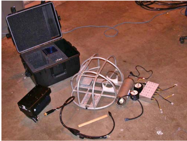
Figure 1. DIDSON components including Pelican case for DIDSON (black device). Also shown is cylindrical battery pressure housing, two battery packs, charger, deck download cable, and protective metal cage. Long (50 ft) underwater cable not shown. Ruler (12 in.) shown for scale.
