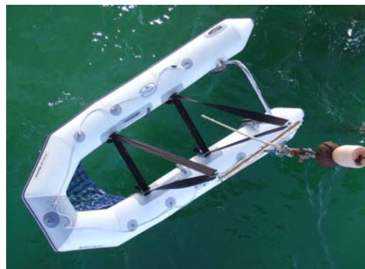
Figure 2. AUV lifting cradle (a) floating on the water with slack given to the support straps (b); and lifted from the water to recover the AUV (c).
