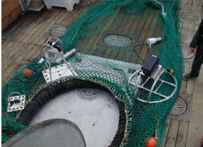
Figure 4. DIDSON and video camera mounting on bottom trawl.
