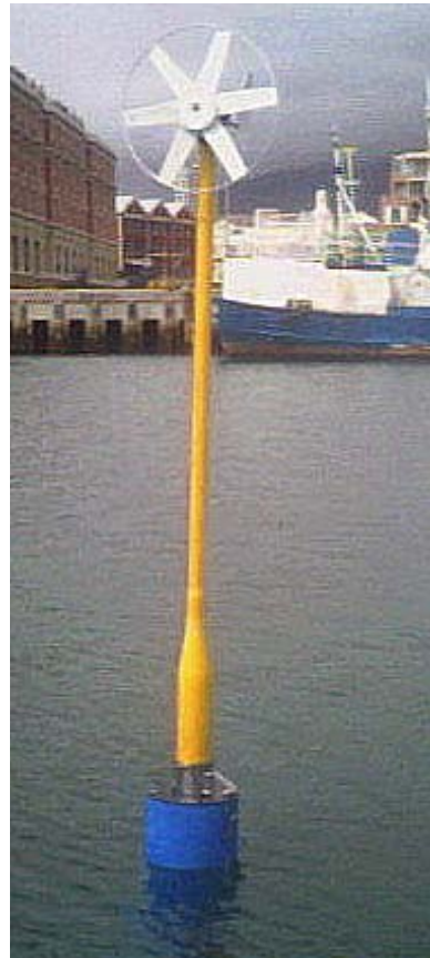
Figure 1. Autonomous data buoy for near-shore ecosystem investigations.
