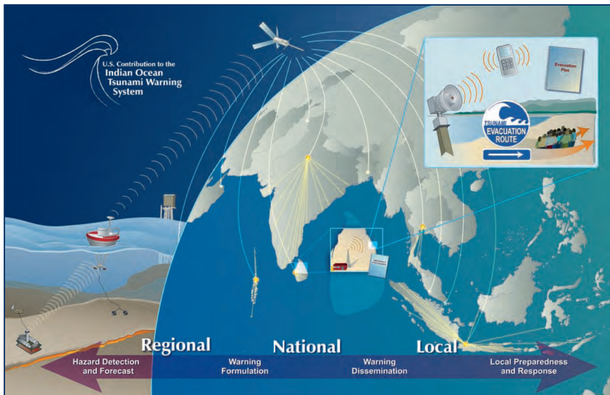
Figure 1-1. Overview of an End-to-End Tsunami Warning System
