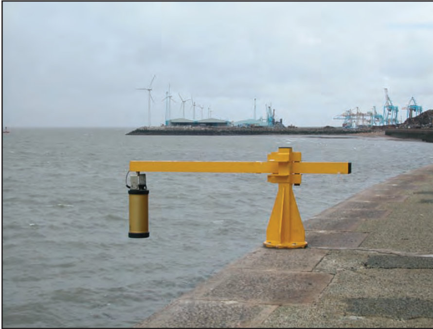
Figure 3-20b. OTT Kalesto Radar Tide Gage at a Test Installation, Liverpool, England (Source: IOC Manual of Sea Level Measurement and Interpretation, Vol. 4, 2006)
