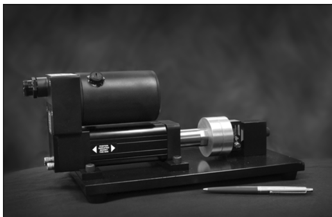
Figure 1. Cyclical Compression Tester device for evaluating orthosis materials used in therapeutic footwear.
