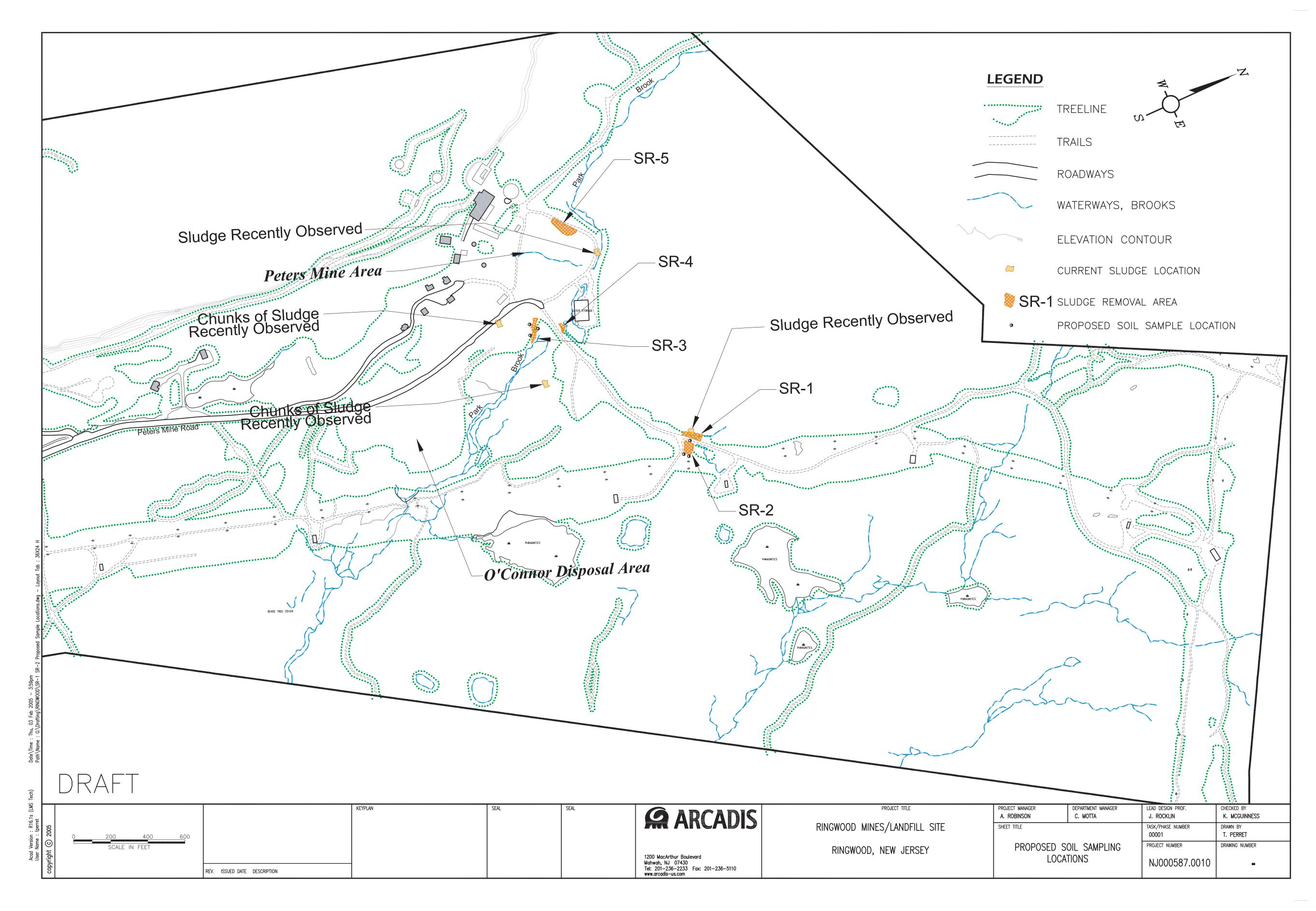
Figure 6: Proposed Soil Sampling Locations and Sludge Removal Areas
