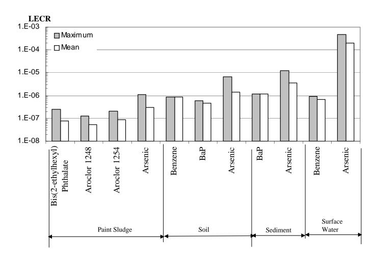
Figure 7: Calculated LECR from Exposures to Contaminants detected in paint sludge, Soil, Sediment and Surface Water
