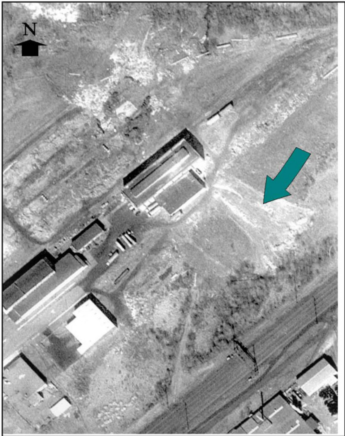
Figure 4. Zonolite/W.R. Grace site. Aerial photograph taken in 1970 showing windblown deposits of vermiculite
