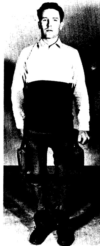
Pneumatic lever anti-g suit designed by Harold Lamport
